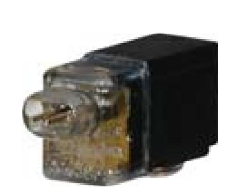
U04 with integrated upward 90° connector
