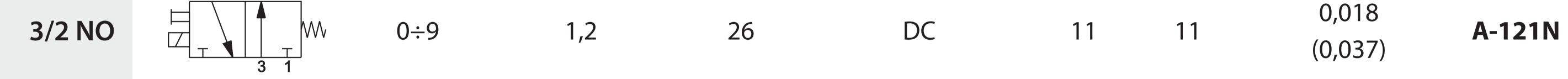
Microvalves Ø 1,5 for direct current coils 2,5 W
